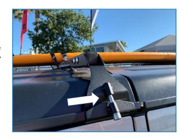
4) Now tighten down all 3/8" Hex Nuts from Step 1 using your Adjustable Wrench. Tighten to compress lock washer. The crossbar should fit tight within the bracket without wiggle.
