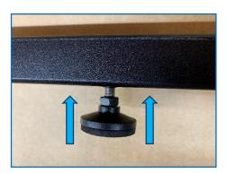
2) Now install the (4) to (6) 1.5" threaded feet all the way into the (2) 51" crossbars. To do so, lower the hex nut on the feet all the way to the pad. Thread entire piece upward into bar all the way (but still loose). Do not tighten. [You are allowing the feet to clear the top during install – later you will lower them down to the roof]
