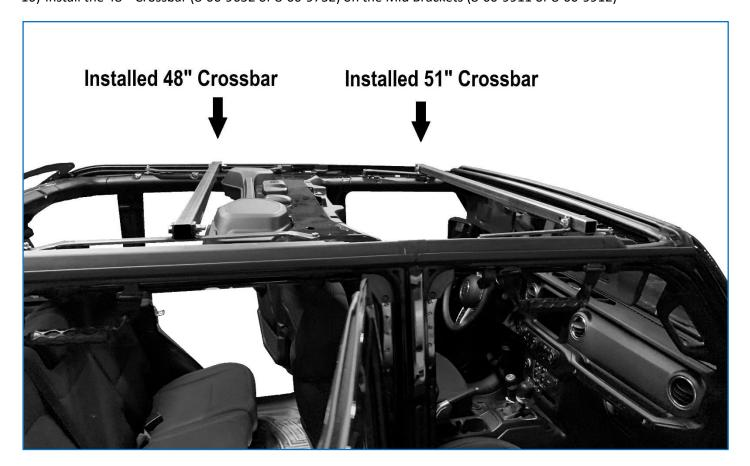
The O'Land Crossbars come with a series of threaded holes on the bottom that allow for the weight distribution feet to be used on the hard top (not used on soft top configuration here). These same holes allow user to mount just about anything to the underside of the crossbar (e.g. light switch panel, CB Radio, etc.). Please see our website for updates and kits available.
