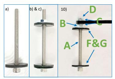
10) Follow Steps 4-7 (as above) to secure brackets. See below for Bolt / Bracket Positions ✓ HAND TIGHTEN ONLY!□ DO NOT USE DRILL GUNOR IMPACT WRENCH!
